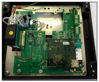
CONNECTING POWER... The TS2020R terminal should be connected using 3A 240V PVC sheathed cable, from the internal fused terminal block, to an easily accessible isolating device as follows:-
