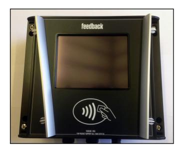
The front comes off but is secured at the bottom edge by plastic straps. Therefore carefully remove the front by lifting upwards and outwards from the top edge.
