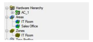
To add a Zone, click on the Add Zone link in the navigation window. Give it a Name and Description as required. drag and drop the required readers into the New Zone window and designate them as either In or Out readers. Click on OK.
