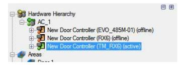
After a door has been added it must be configured to suit the hardware connected to it. To carry out any editing of the parameters, right click on the controller in either the **Hardware Hierarchy** or on the **Structure Panel**.
