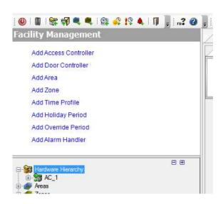
To add an Access Controller manually, click on the Add Access Controller link in the navigation window. Give it a **Name** and **Description**. To make it active on the system, tick the **Active** checkbox.
