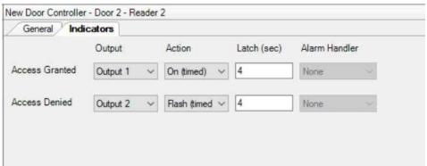
Alternatively, these events can initiate an alarm handler instead of using an Output, by selecting the appropriate handler from the drop-down list.
